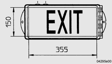
Emergency exit sign
